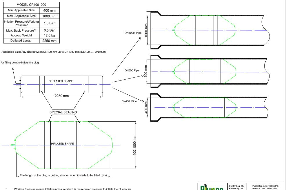
: Working Pressure means Inflation pressure which is the required pressure to inflate the plug by air.
