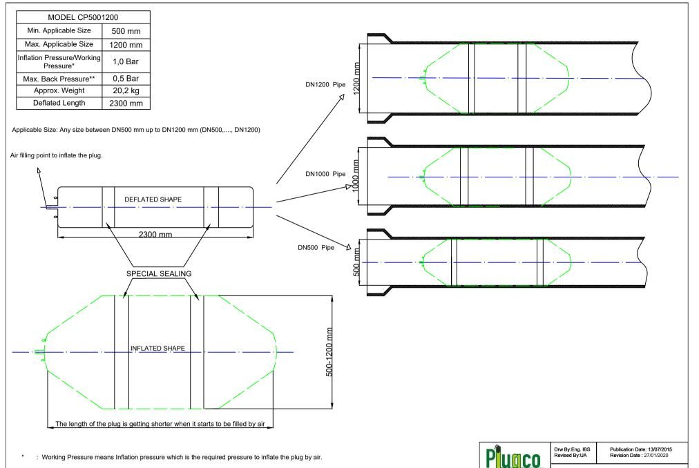
$^{\star\star}$   $\,\,$  : Back Pressure refers to the  $\,$  pressure  $\,$  which pushes the plug and forces it to move inside the pipeline.
