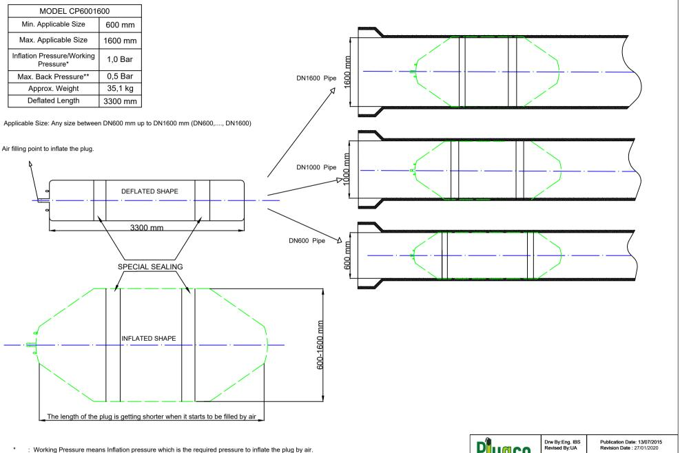
\*\* : Back Pressure refers to the pressure which pushes the plug and forces it to move inside the pipeline.
