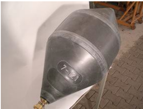
9. Now, the cushion has been inflated. While reaching the maximum pressure of 1 bar, the safety valve will open automatically and blow-off the air.
