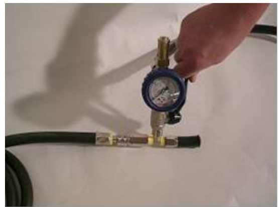
10. Close the ball valve of the safety fitting and break the air flow until the safety valve will close
