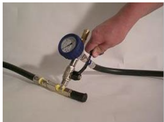
6. Open the ball valve of the safety fitting slowly . Now the air can run into the cushion
