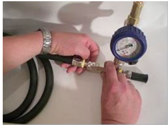
2. Couple the pre-pressure hose on the left coupling (yellow) of the safety fitting and lock the connection by turning the screw retention. Please ensure, that the ball valve always stands transverse to the flow direction.
