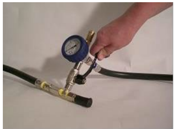
12. Now open again the ball valve for a short time, which the pre pressure is able to flow out.
