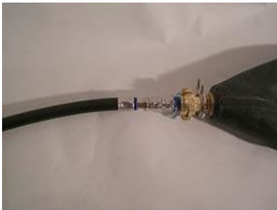
3. Couple the blue-marked coupling of the filling hose on the nipple of the Conical Plug and lock the connection by turning the screw retention.
