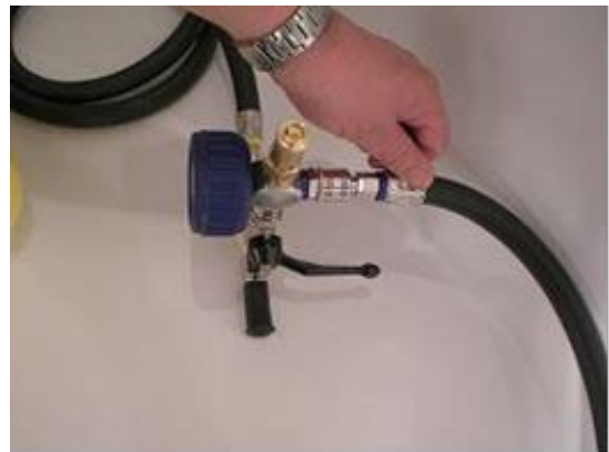
4. Connect the other side of the filling hose (nipple) with the blue-marked coupling on the bottom side of the safety fitting and lock the connection by turning the screw retention.
