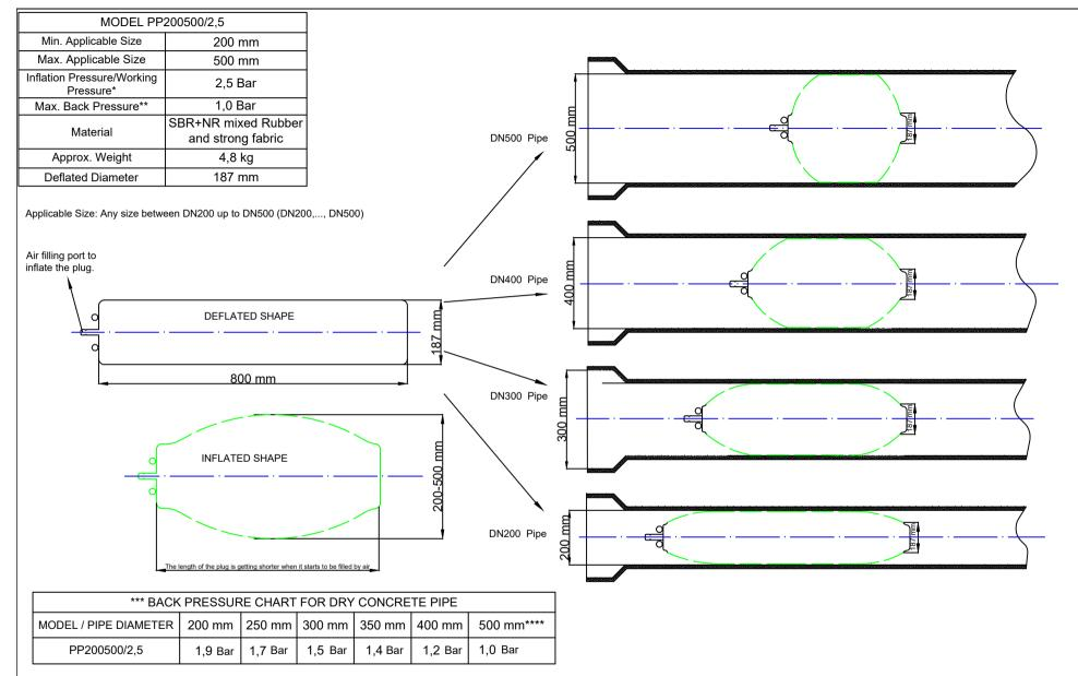
\* : Working Pressure means Inflation pressure which is the required pressure to inflate the plug by air.
